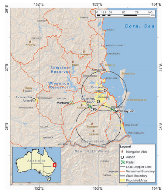
Figure 1. Map of Southeast Queensland region targeted for the Queensland CSRP field effort and associated facilities and landmarks. The 30-degree beam crossing angle dual-Doppler lobes are overlaid in black.
