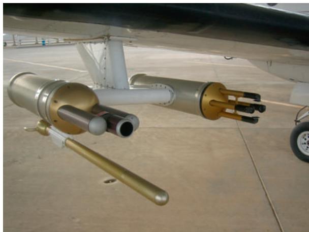
Figure 3: FSSP (left) and 2D-S (right) mounted under the right wing.
