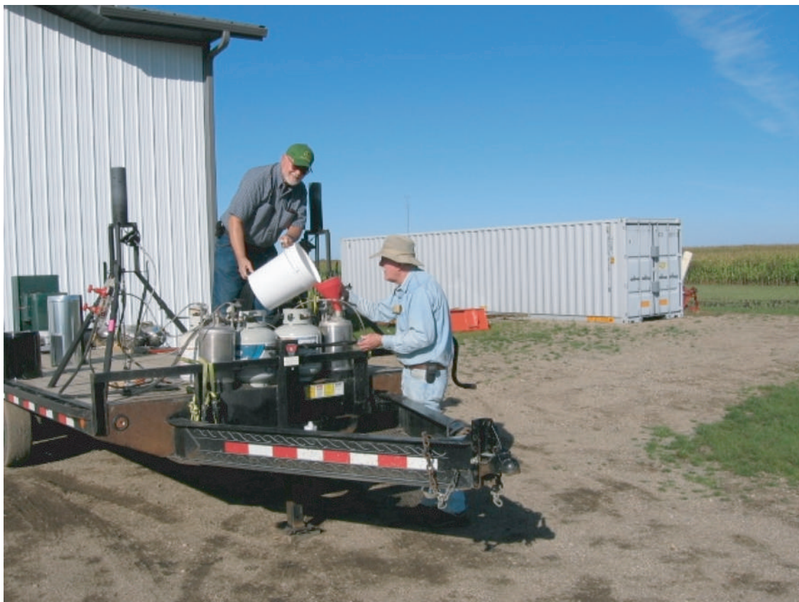
Figure 2. The flatbed trailer used for mobile releases of Agl during generator and solution comparison tests parked by the ICE facility. Two black MSU Skyfire generators are in the foreground with seeding solution being poured into a stainless steel tank by A. Super (left) and J. McPartland. The dark green WMI generator is mounted at trailer's rear. A silver wind shield used with a Skyfire is in front of the WMI unit. The extreme flatness of the terrain is evident; note the corn field in the background (right) of the photo. (Photograph by A. Super.)
