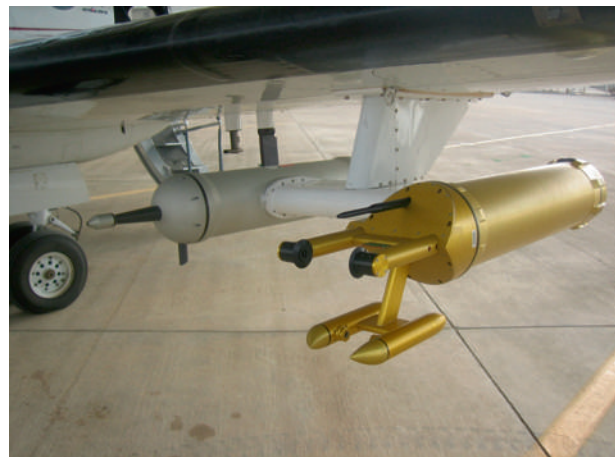
Figure 4: PCASP (left) and CIP/CDP/LWC combination probe (right) mounted under the left wing.
