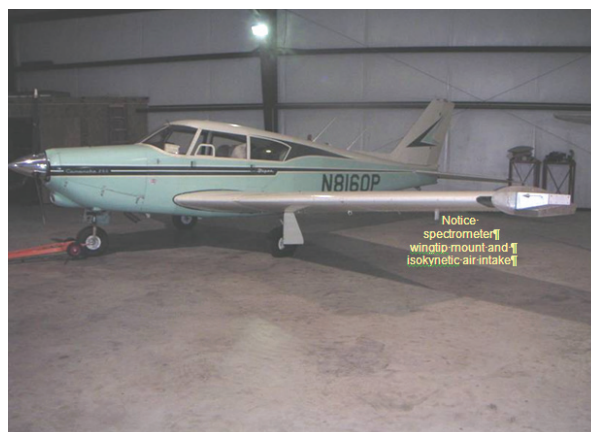
Fig. 4. Piper Comanche 260B, Equipped with Two Wingtip Mounted Spectrometers
