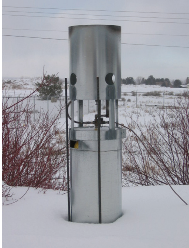
Fig. 5. Ground Based, Manually Operated Silver Iodide Generator
