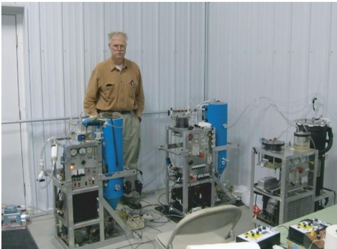
Figure 1. The three AINCs. from left to right are: Unit 1 tested at the CSU ICC during 1994; Unit 3, newly constructed for the Snowy Hydro program in Australia by J. Heimbach (pictured); and Unit 2, the WMI counter. (Photograph by A. Super)
